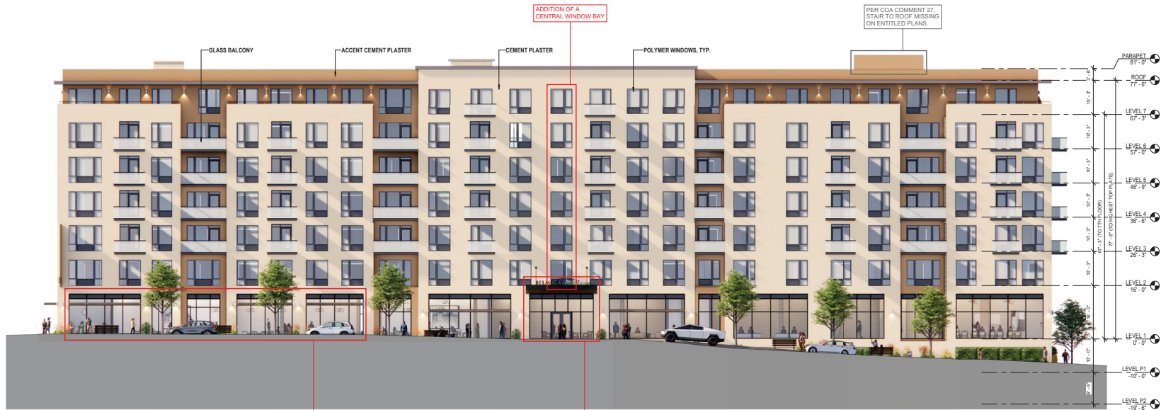
1 PROPOSED NORTH ELEVATION 3/32" = 1'-0" *WINDOW SIZE AND POSITIONS HAVE BEEN ADAPTED TO MEET INTERIOR UNIT LAYOUT.
